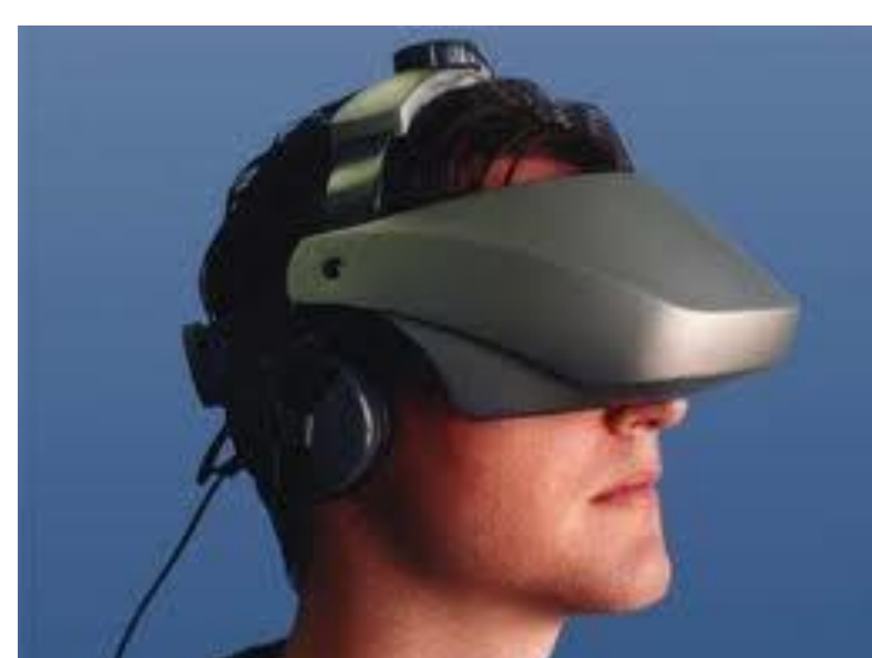
Head-Mounted Display (HMD)
